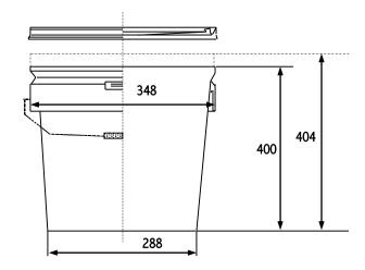
Measurements in millimetres
